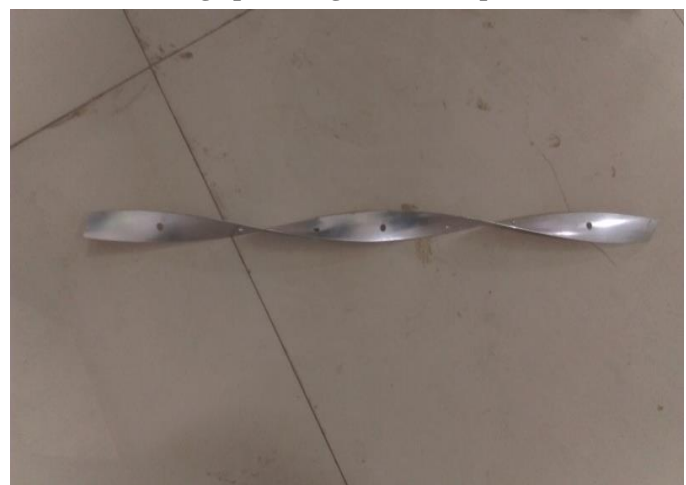
Fig2. Twisted tape with drilled holes
