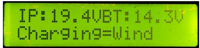
Fig. 8 Message Displayed on LCD When Input Voltage is Above threshold voltage
