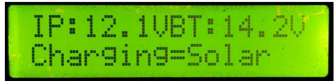
Fig. 7 Message Displayed on LCD when input voltage is below threshold voltage.
