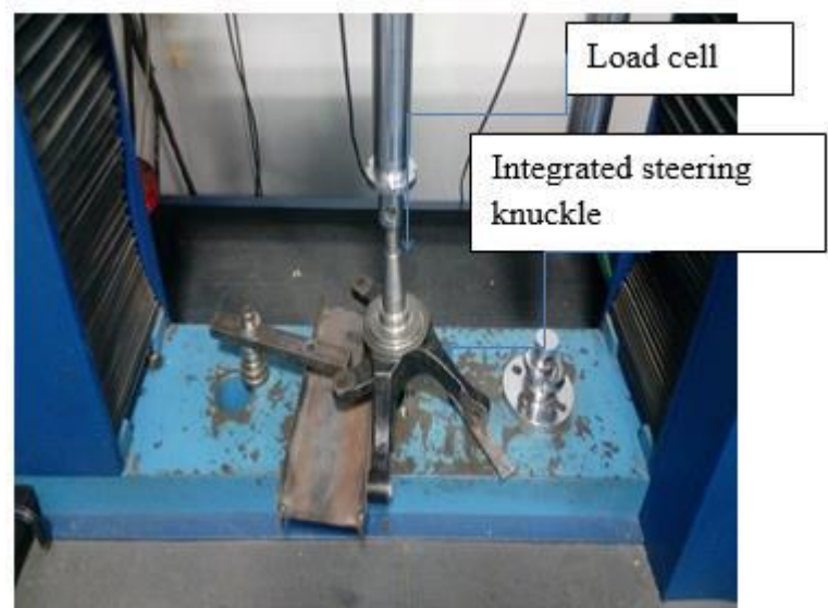
Figure 7: Experimental set up of integrated steering knuckle for lateral test
