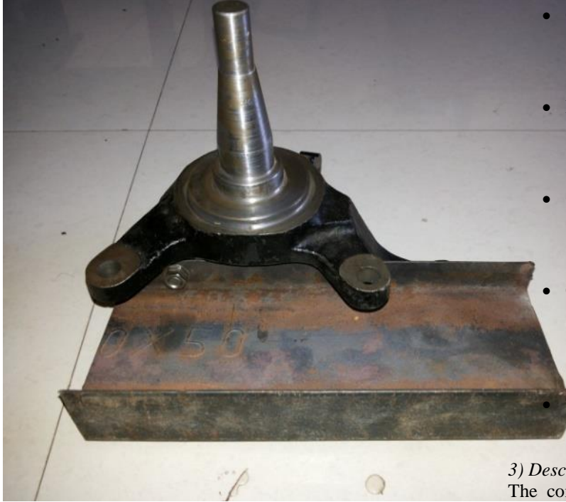
Figure 6: Final prototype of integrated steering knuckle with fixture plate
