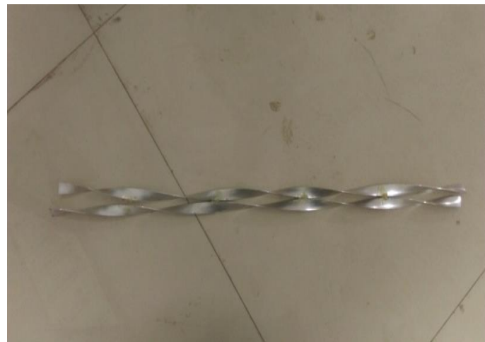
Fig3. Twisted tape with clockwise-anticlockwise direction
