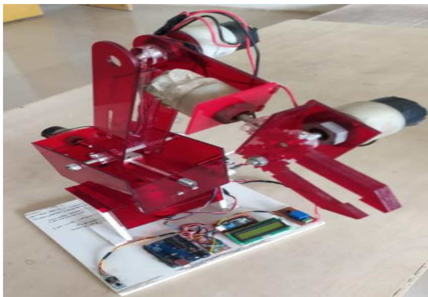
Figure B.2.2.3.i: To Design and Develop Prototype of Industrial Cobot
