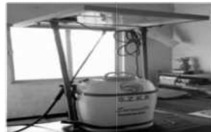
Fig.4 Field evaluation of trolley based solar sprayer
