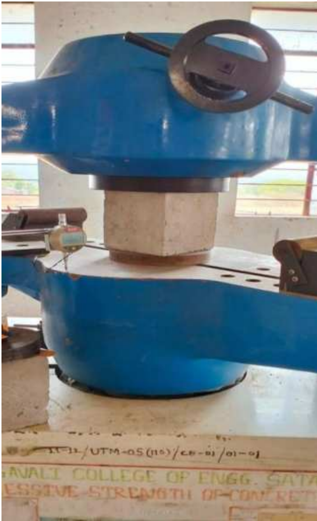
Cube Testing On UTM
