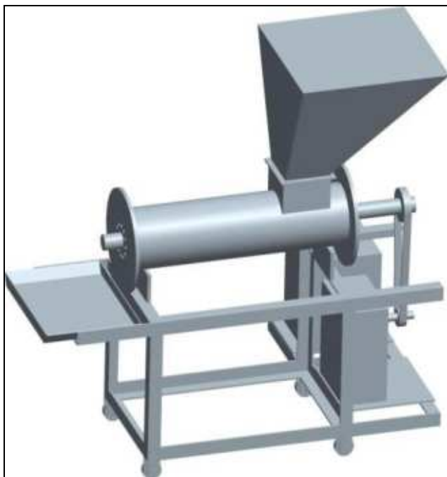
Fig. 2. Pellet machine for handling of biogas slurry
