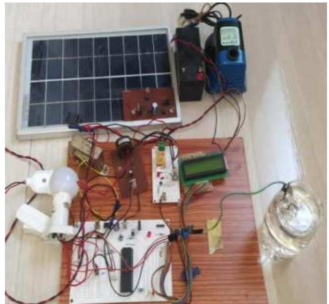
Fig. 5. Pictorial representation of the Automatic Drip-Irrigation System.
