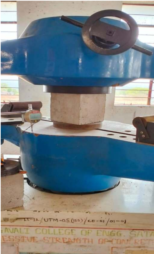
Cube Testing On UTM
